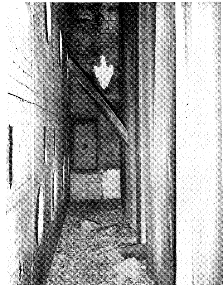
Figure 3 and 4. Two views of fallen pieces of shattered HK-40 tubes lying in catalyst and rubble on the floor of the reformer.
