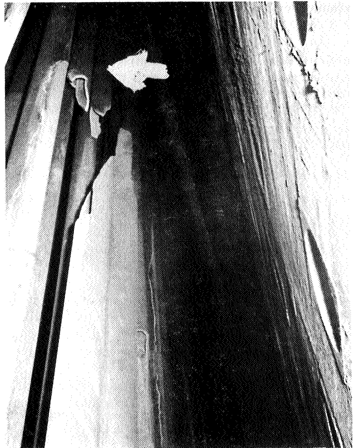
Figure 1 and 2. Two views of the hanging remains of severed tubes, with the fractured ends indicated by the arrows.
